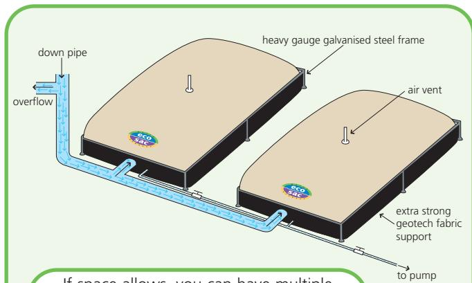
If space allows, you can have multiple bladders installed side by side or end to end, with pipes connecting them so that they can all fill at the same time. When all the bladders are full any excess water is diverted straight to the existing stormwater drain.
